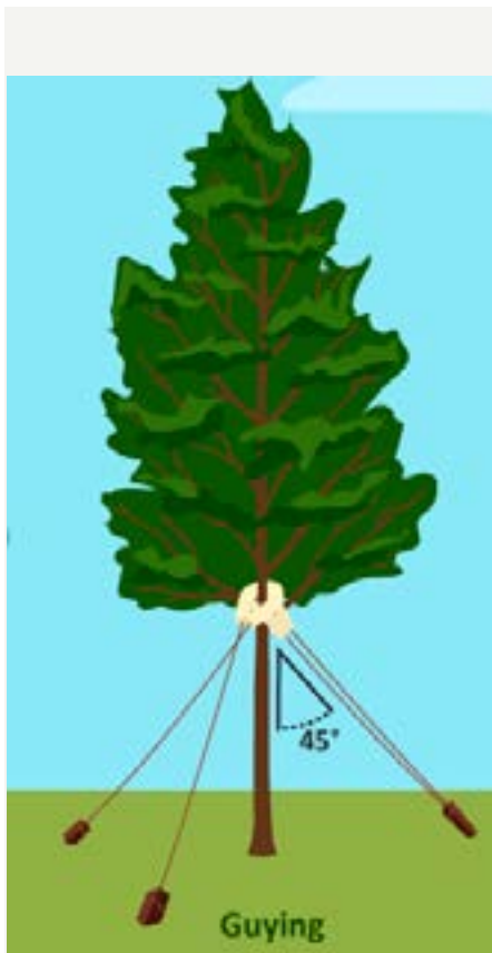
Figure 4 - Correct Guying Method.
